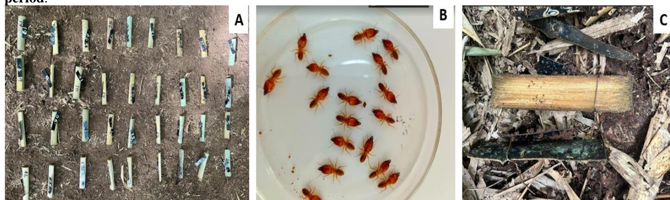
Figure 3: a) layout of samples in the field, b) M. bellicosus termites, c) samples at the end of the test period.
