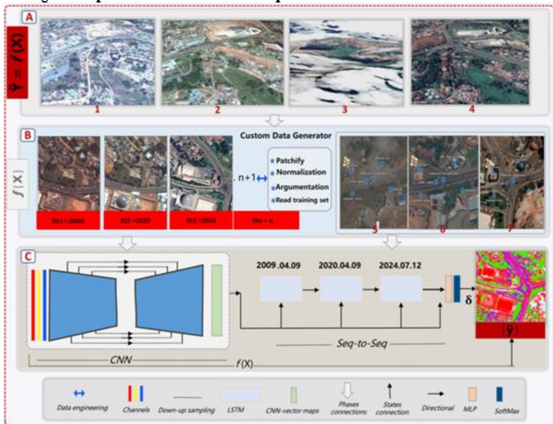
Figure 1: Comprehensive Land Cover Workflow Using Multisource Data and Sentinel-2 Imagery to Distinguish Impervious Roads from Built-up Areas.
